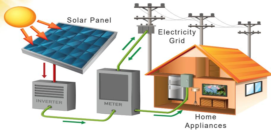
Figure 10: On -Grid Solar System
