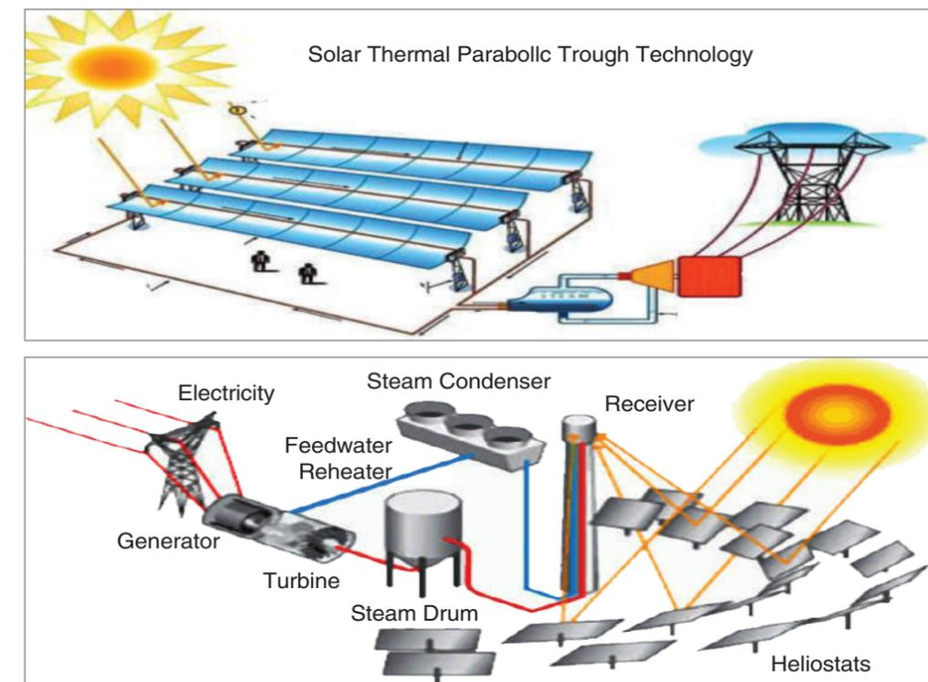
Figure 7: Solar Thermal Energy
